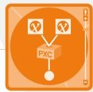
A network connects to the AMS-IX platform through a Photonic Cross Connect (PXC). If one connection fails, the PXC can move the network's traffic to the backup connection within milliseconds.
